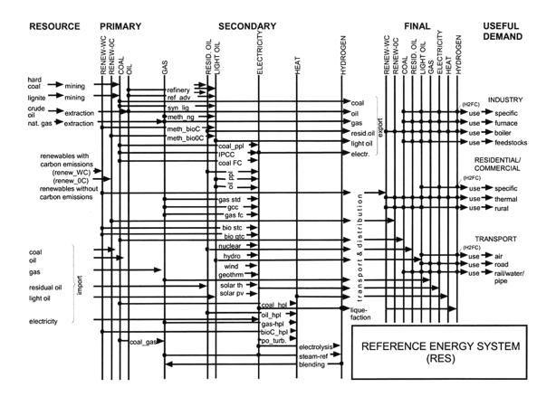
Figure 2.3. – Reference Energy System [Nak00], used as input for the MESSAGE model.
